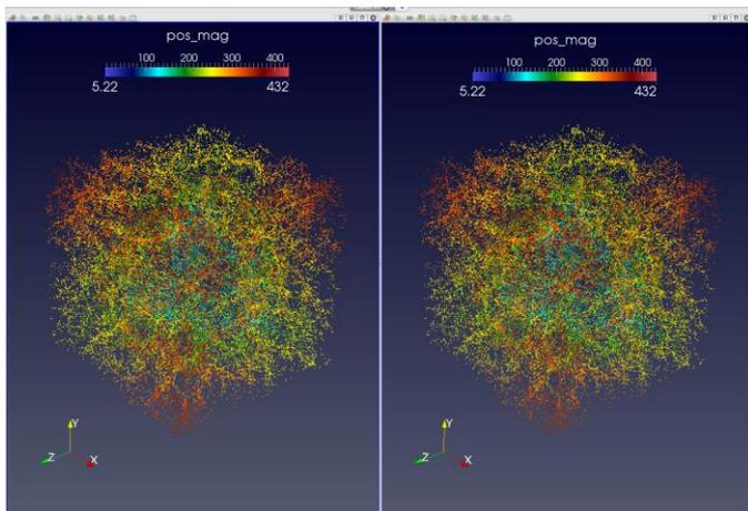
Visual comparison of halos computed by the original HACC algorithms (left) and the PISTON algorithms (right). The results are equivalent, but are computed much more quickly on the GPU using PISTON.
